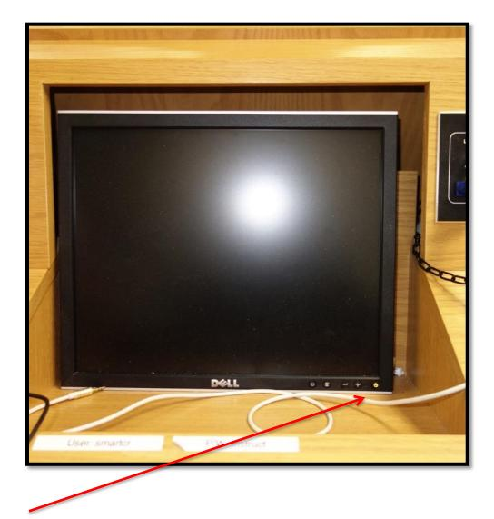
In the lower right corner of the monitor is a button with a light. If the light is "amber" the monitor is on and waiting for the computer to start. If the light is off, push the button to turn on the monitor. When the PC is on, the light will turn green.
