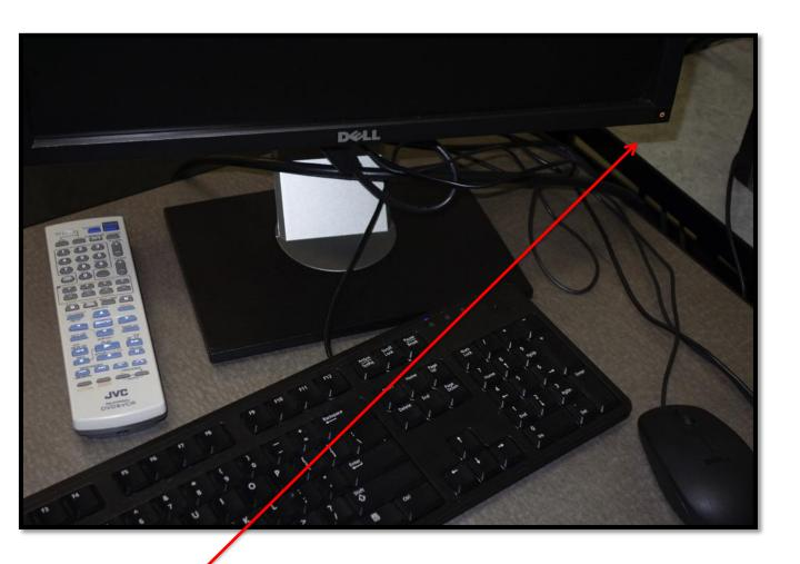
In the lower right corner of the monitor is a button with a light. If the light is "amber" the monitor is on and waiting for the computer to start. If the light is off, push the button to turn on the monitor. When the PC is on, the light will turn green.
